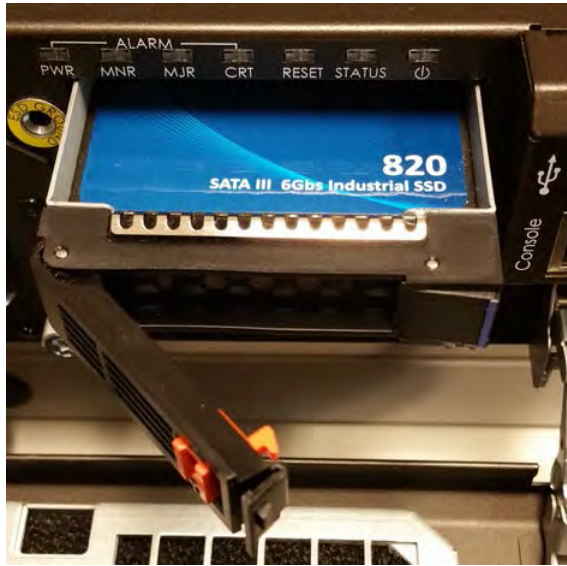
FIGURE 3 An open disk tray
