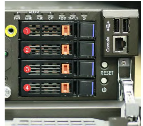
FIGURE 2 Disk trays on the front panel of the controller
